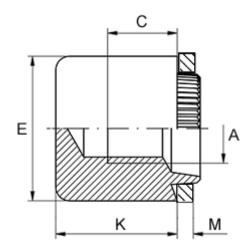
Female thread A = M3Height K = 9.0Min thread length C = 3.0Outer diameter E = 8.0Plate thickness = 1.4 to 1.6
